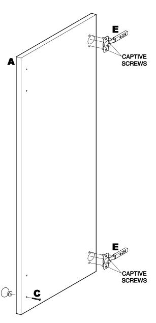
**2.1** Align rear plugs and hinge cup on Hinge (E) with recesses in Door (A), then press Hinge onto Door until flush. Tighten captive screws to expand plugs and secure Hinge in place.
