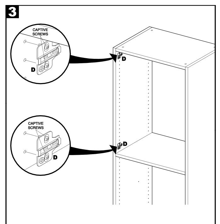
**3.1** Align rear plugs on Hinge Plates (D) with two upper and lower holes in Tower, then press Hinge Plates onto Tower until flush. Tighten captive screws to expand plugs and secure Hinge Plates in place.
