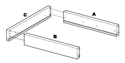
**3.1** Align Wood Dowels in Front Drawer Panel (A) and Rear Drawer Panel (B) with holes in one Side Drawer Panel (C), and press components together until flush.
