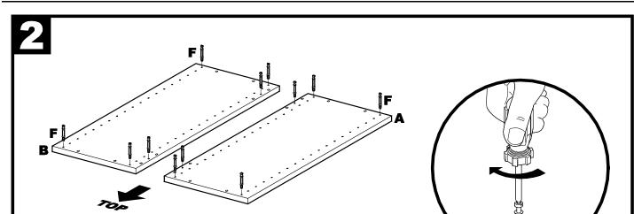
2.1 Install one Cam Post (F) into each of the sic holes on Left Side Panel (A) and Right Side Panel (B). Tighten until Cam Posts are seated against Side Panels.
