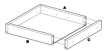
**5.1** Align Side Drawer Panel (C) with Wood Dowels in Front Drawer Panel (A) and Rear Drawer Panel (B) and press Side Drawer Panel (C) onto assembled components until flush.
