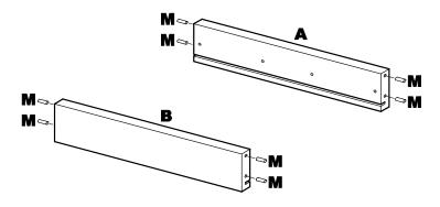
2.1 Insert Wood Dowels (M) into holes in ends of Front Drawer Panel (A) and Rear Drawer Panel (B).
