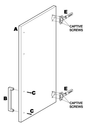
**2.1** Align rear plugs and hinge cup on one Hinge (E) with recess in Door (A), then press Hinge onto Door until flush. Tighten captive screws to expand plugs and secure Hinge in place. Repeat for remaining Hinges.
