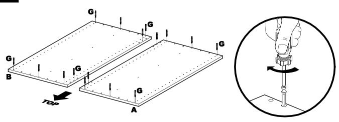
2.1 Install one Cam Post (G) into each of the eight holes on Left Side Panel (A) and Right Side Panel (B). Tighten until Cam Posts are seated against Side Panels.
