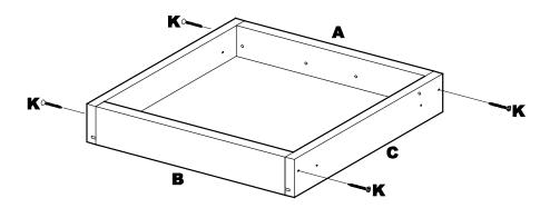
**6.1** Secure Side Drawer Panels (C) to Front Drawer Panel (A) and Rear Drawer Panel (B) using 1.0" Drawer Side Screws (K).
