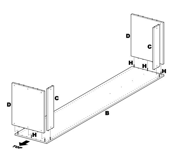
**4.1** Assemble Set Shelves (D) and Rear Hanging Cleats (C) onto Right Side Panel (B) by sliding the Shelves and Cleats onto Cam Posts (H) on Right Side Panel. BE SURE dowel pins in Shelves and Cleats engage drilled holes in Right Side Panel, and all parts are pressed flush against Right Side Panel.
