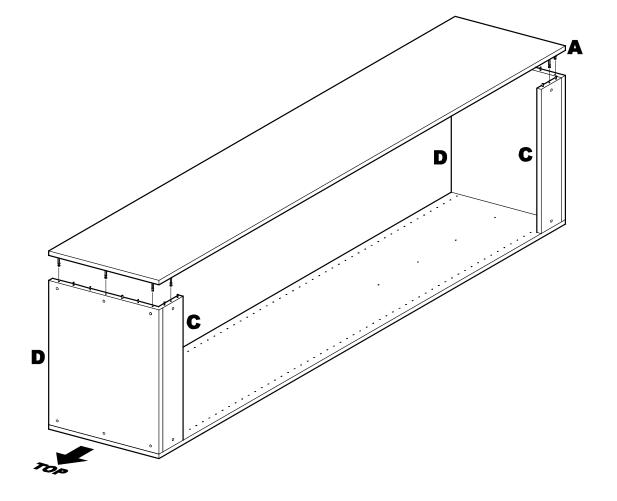
**5.1** Install Left Side Panel (A) onto assembled Set Shelves (D) and Rear Hanging Cleats (C). BE SURE dowel pins in Shelves and Cleats engage drilled holes in Side Panel, and Side Panel is pressed flush against Set Shelves and Cleats.
