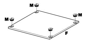
3.1 Insert four Knock-in Housings (M) into recesses in Adjustable Set Shelf (F). Gently tap each Knock-in Housing (M) into Adjustable Set Shelf (F) using a rubber mallet until lip on Knock-in Housing is flush with surface of Shelf.
