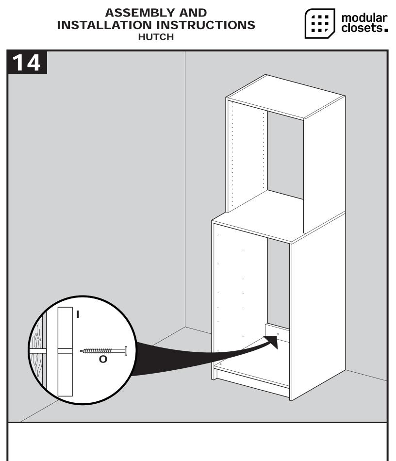
**14.1** Secure Rear Hanging Cleats (I) to studs using six 2.5" screws (O).
