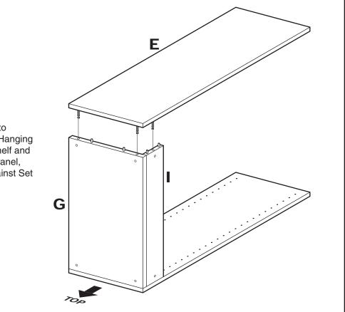
10.1 Install Upper Left Side Panel (E) onto assembled Set Shelf (G) and Rear Hanging Cleat (I). BE SURE dowel pins in Shelf and Cleat engage drilled holes in Side Panel, and Side Panel is pressed flush against Set Shelf and Cleat.
