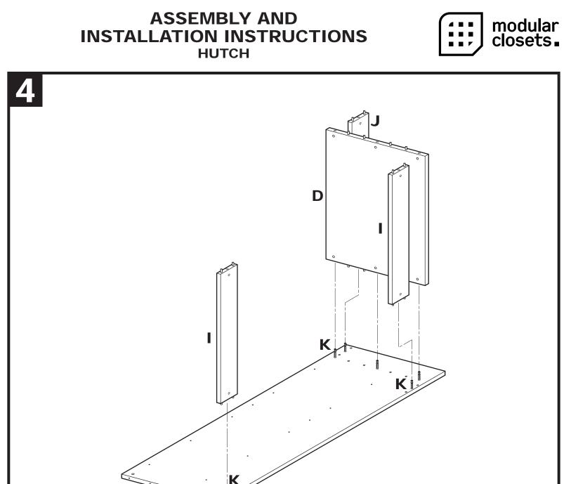
4.1 Assemble Base Set Shelf (D), Rear Hanging Cleats (I) and Toe Kick (J) onto Base Right Side Panel (B) by sliding the Shelves, Cleats and Toe Kick onto Cam Posts (K) on Right Side Panel. BE SURE dowel pins in Shelves, Cleats and Toe Kick engage drilled holes in Right Side Panel, and all parts are pressed flush against Panel.
