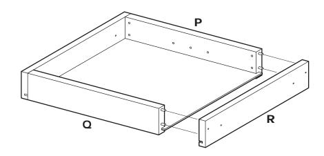
**19.1** Align Side Drawer Panel (R) with Wood Dowels in Front Drawer Panel (P) and Rear Drawer Panel (Q) and press SIde Drawer Panel (R) onto assembled components until flush.
