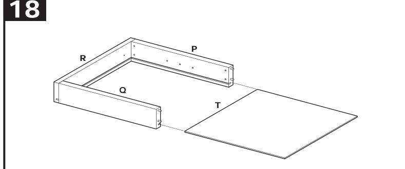
NOTE: Be sure to install Drawer Bottom (T) with finished side facing up.
