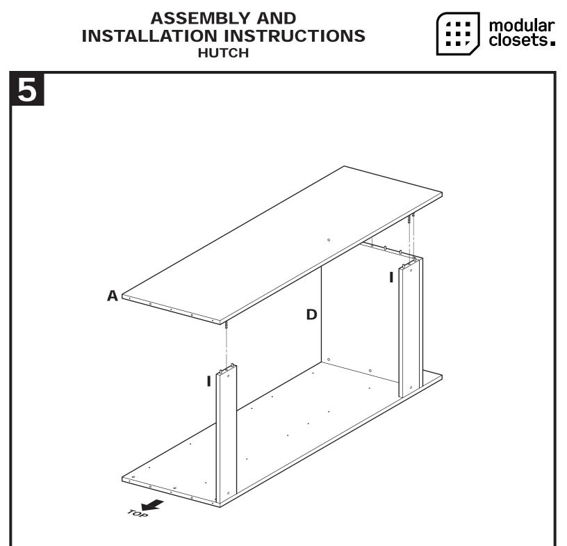
5.1 Install Base Left Side Panel (A) onto assembled Set Shelf (D), Rear Hanging Cleats (I) and Toe Kick (J). BE SURE dowel pins in Shelf, Cleats and Toe Kick engage drilled holes in Side Panel, and Side Panel is pressed flush against Set Shelf, Cleats and Toe Kick.
