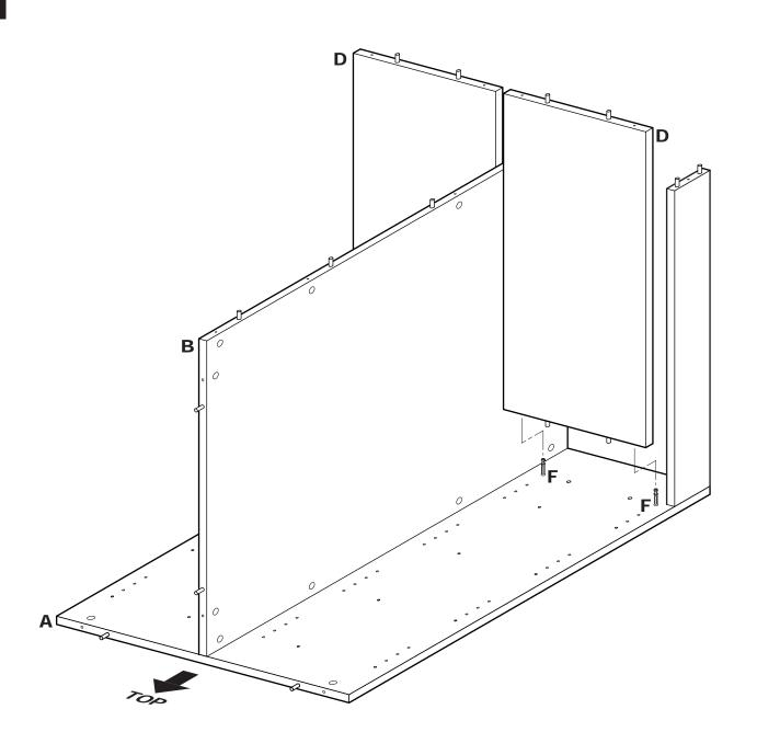
**5.1** Assemble two Fixed Shelves (D) onto Side Panel (A) by sliding the Shelves onto the Cam Posts (F) on Side Panel (A). BE SURE dowel pins in Shelves engage drilled holes in Side Panel, and all parts are pressed flush against Side Panel.
