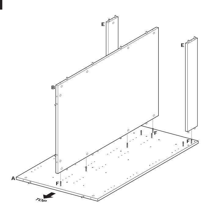
**4.1** Assemble Vertical Panel (B) and two Cleats (E) onto Side Panel (A) by sliding the Vertical Panel and Cleats onto the Cam Posts (F) on Side Panel (A). BE SURE dowel pins in Vertical Panel and Cleats engage drilled holes in Side Panel, and all parts are pressed flush against Side Panel.
