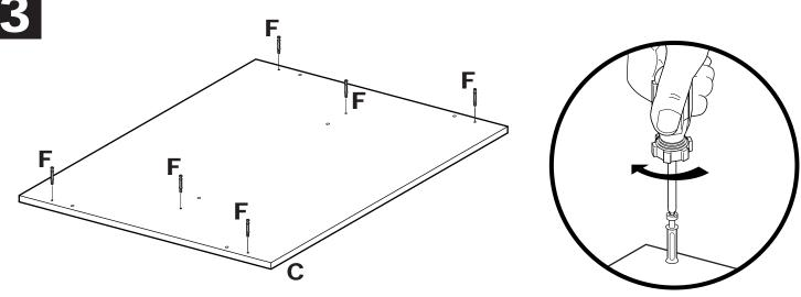
**3.1** Install one Cam Post (F) into each of the six holes on Top Panel (C). Tighten until Cam Posts are seated against Top Panel.
