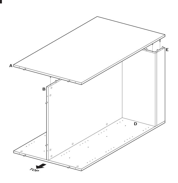
6.1 Install second Side Panel (A) onto assembled Vertical Panel (B), Fixed Shelves (D) and Cleats (E). BE SURE dowel pins in Vertical Panel, Shelves and Cleats engage drilled holes in Side Panel, and Side Panel is pressed flush against Panel, Shelves and Cleats.
