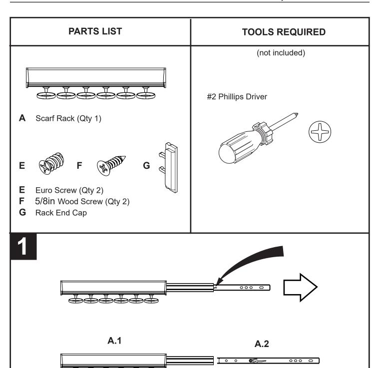
**NOTE:** Each Scarf Rack is shipped assembled. To separate, lift the plastic catch on the Panel Side and pull the slide out of the Rack Side
