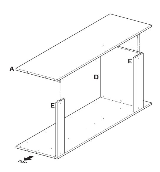
**5.1** Install Base Left Side Panel (A) onto assembled Set Shelf (D), Rear Hanging Cleats (E) and Toe Kick (F). BE SURE dowel pins in Shelf, Cleats and Toe Kick engage drilled holes in Side Panel, and Side Panel is pressed flush against Set Shelf, Cleats and Toe Kick.
