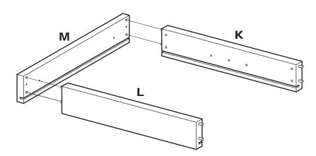
**11.1** Align Wood Dowels in Front Drawer Panel (K) and Rear Drawer Panel (L) with holes in one Side Drawer Panel (M), and press components together until flush.
