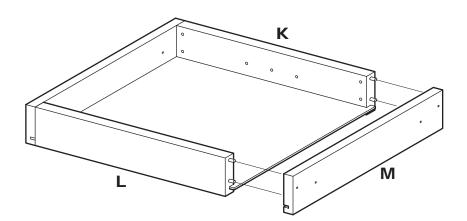
**13.1** Align Side Drawer Panel (M) with Wood Dowels in Front Drawer Panel (K) and Rear Drawer Panel (L) and press Side Drawer Panel (M) onto assembled components until flush.
