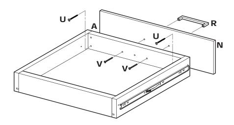
**NOTE:** DO NOT overtighten Screws (U) or surface of Drawer Front (N) may become dimpled.
