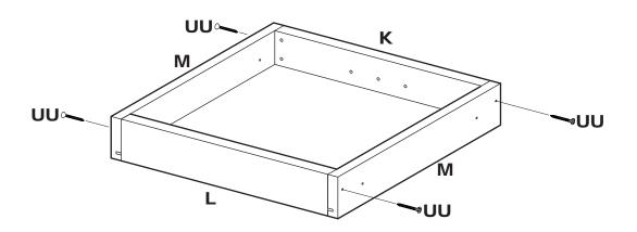
**14.1** Secure Side Drawer Panels (M) to Front Drawer Panel (K) and Rear Drawer Panel (L) using 1.5" Drawer Side Screws (UU).
