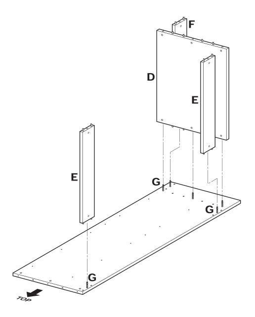
4.1 Assemble Base Set Shelf (D), Rear Hanging Cleats (E) and Toe Kick (F) onto Base Right Side Panel (B) by sliding the Shelves, Cleats and Toe Kick onto Cam Posts (G) on Right Side Panel. BE SURE dowel pins in Shelves, Cleats and Toe Kick engage drilled holes in Right Side Panel, and all parts are pressed flush against Panel.
