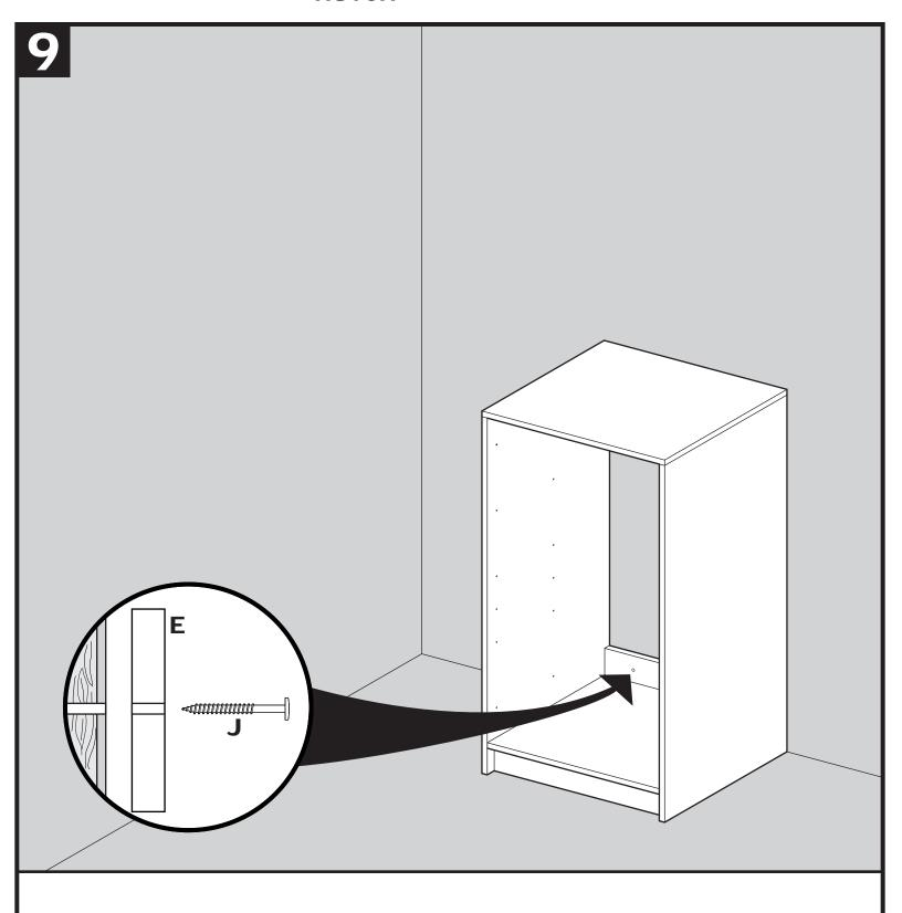
**9.1** Secure Rear Cleats (E) to studs using six 2.5" screws (J).
