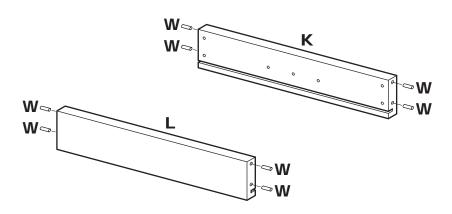
10.1 Insert Wood Dowels (W) into holes in ends of Front Drawer Panel (K) and Rear Drawer Panel (L).
