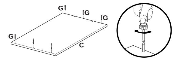
2.1 Install one Cam Post (G) into each of the 6 holes on Base Top Shelf (C). Tighten until Cam Posts are seated against Top Shelf.
