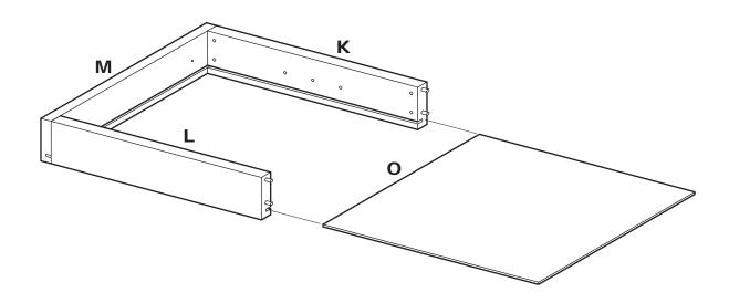
NOTE: Be sure to install Drawer Bottom (0) with finished side facing up.
