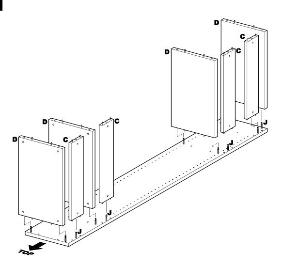
**3.1** Assemble Set Shelves (D) and Rear Hanging Cleats (C) onto Right Side Panel (B) by sliding the Shelves and Cleats onto the Cam Posts (J) on Side Panel. BE SURE dowel pins in Shelves and Cleats engage drilled holes in Side Panel, and all parts are pressed flush against Side Panel.
