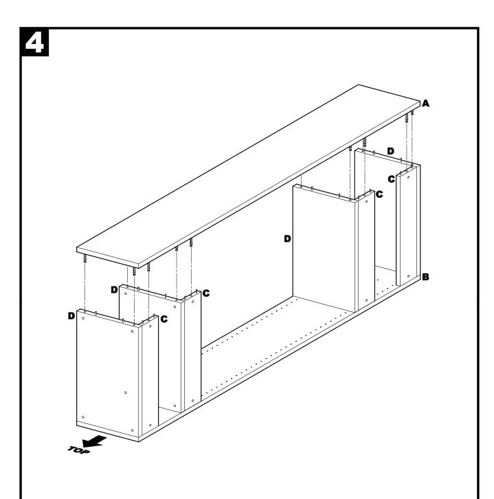
**4.1** Install Left Side Panel (A) onto assembled Set Shelves (D) and Rear Hanging Cleats (E). BE SURE dowel pins in Shelves and Cleats engage drilled holes in Side Panel, and Side Panel is pressed flush against Set Shelves and Cleats.
