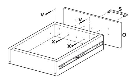
NOTE: DO NOT overtighten Screws (W) or surface of Drawer Front (O) may become dimpled.
