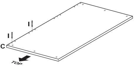
**3.1** Install one Cam Post (I) into each of the 2 holes on Left Leg (C) Tighten until Cam Posts are seated against Leg.
