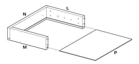
**NOTE:** Be sure to install Drawer Bottom (P) with finished side facing up.
