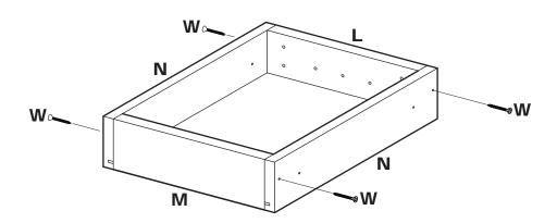
16.1 Secure Side Drawer Panels (N) to Front Drawer Panel (L) and Rear Drawer Panel (M) using 1.5" Screws (W).
