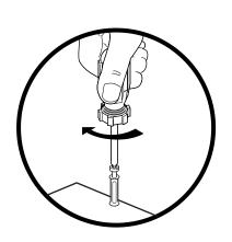
**8.1** Install one Cam Post (I) into the hole on Right Side Panel (B). Tighten until Cam Post is seated against Side Panel.
