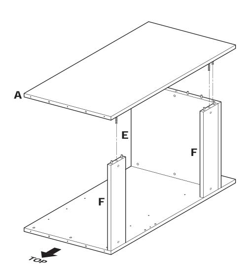
**5.1** Install Base Left Side Panel (A) onto assembled Set Shelf (E), Rear Hanging Cleats (F) and Toe Kick (G). BE SURE dowel pins in Shelf, Cleats and Toe Kick engage drilled holes in Side Panel, and Side Panel is pressed flush against Set Shelf, Cleats and Toe Kick.
