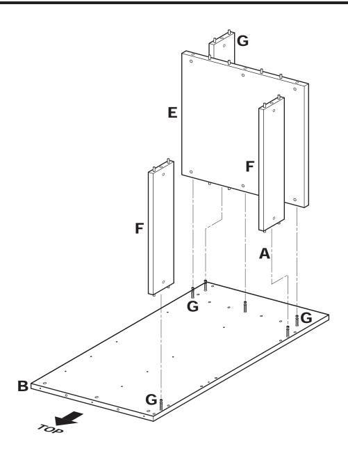
4.1 Assemble Set Shelf (E), Rear Cleats (F) and Toe Kick (G) onto Right Side Panel (B) by sliding the Shelves, Cleats and Toe Kick onto Cam Posts (I) on Right Side Panel. BE SURE dowel pins in Shelves, Cleats and Toe Kick engage drilled holes in Right Side Panel, and all parts are pressed flush against Panel.
