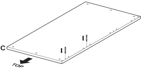
**3.1** Install one Cam Post (I) into each of the 2 holes on Right Leg (C) Tighten until Cam Posts are seated against Leg.
