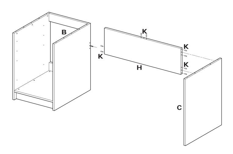
**9.1** Assemble Right Leg (C), Stretcher (H) and Cabinet. BE SURE dowel pins in Stretcher engage drilled holes in Right Leg (C) and Cabinet Side Panel (B) and components are pressed flush.
