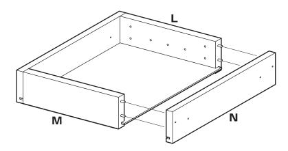
**15.1** Align Side Drawer Panel (N) with Wood Dowels in Front Drawer Panel (L) and Rear Drawer Panel (M) and press Side Drawer Panel (N) onto assembled components until flush.
