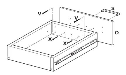
**NOTE:** DO NOT overtighten Screws (V) or surface of Drawer Front (O) may become dimpled.
