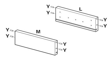
12.1 Insert Wood Dowels (Y) into holes in ends of Front Drawer Panel (L) and Rear Drawer Panel (M).
